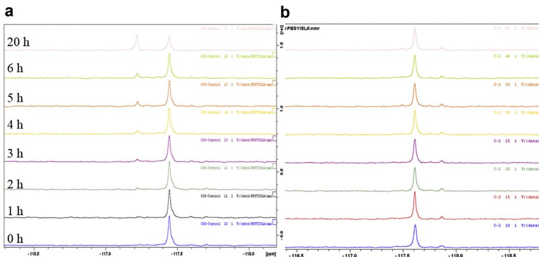
**Fig. 4.**  $^{19}\text{F}$  NMR data presenting the inhibition of MMP-9 by MMP-9 inhibiting NPs. (a) Cleavage of a MMP-9 cleavable peptide (TY-26) by MMP-9 enzyme is represented by disappearing signal at  $-117.5$  ppm and appearance of enzyme degradation product signal at  $-117.2$  ppm, (b) The inhibition of TY-26 cleavage by MMP-9 inhibiting NPs in the presence of MMP-9 enzyme is shown by persistent signal at  $-117.5$  ppm and no any other signals.
