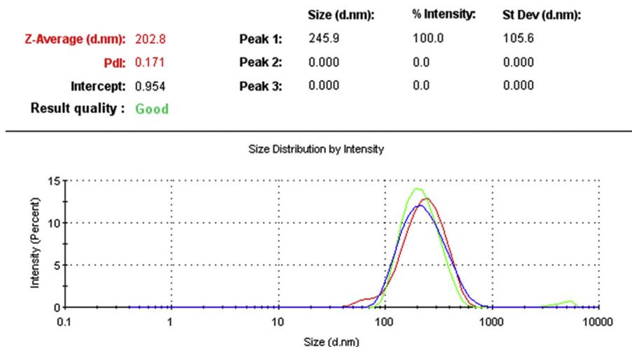
**Fig. 2.** Particle size distribution report of MMP-9 inhibiting nanoparticles obtained by the DLS method. This figure shows three different measurements. The average particle size and Pdl are presented at the top of figure.
