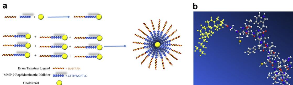
**Fig. 1.** (a) Schematic diagram of the formation of self-assembled MMP-9 inhibiting NPs by amphiphilic peptides. (b) Ball and stick presentation of the MMP-9 inhibiting amphiphilic compound: Cholesterol-CTTHWGFTLCHAIYPRH. Cholesterol is presented as yellow ball and sticks.
