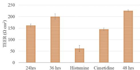
**Fig. 7.** TEER values for *in vitro* BBB prepared by hCMEC/D3 cells seeded at 90,000/inset after 24 h, 36 h, post histamine and post cimetidine treatment, presenting formation of a biological barrier that can be compromised by pharmacological compounds (histamine) and restated by pharmacological agents (cimetidine). Error bar indicate SD (n = 3).
